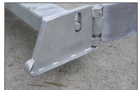
Wide and bent up side skids
