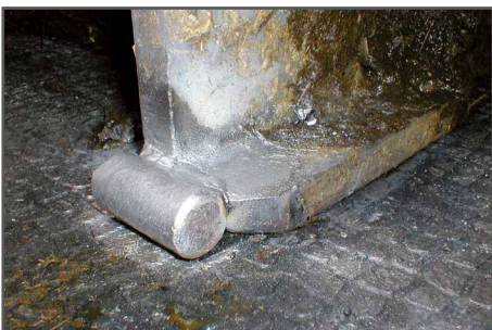
Side skids with round bar and wide bearing
