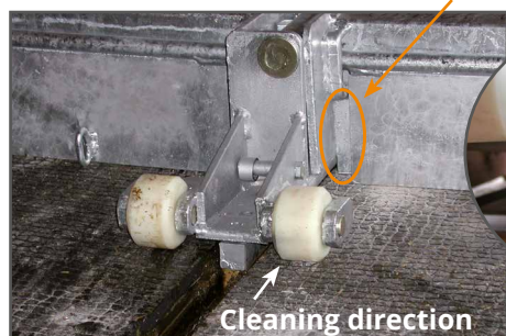
Center bracket rests on wide plastic rolls
