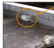
Cam block on main cleaning flap with roller
